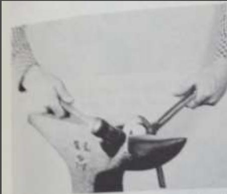
Fig. 29-8. Step 3. Place the tapered end of the branch diagonally over the base of the horn with about one-half inch projecting beyond the spot where it contacts the horn.
