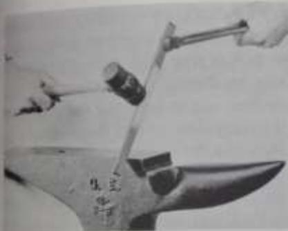
Fig. 29-3. Step 3. Hold the bar at a 45° angle and the tongs parallel to the anvil face.
